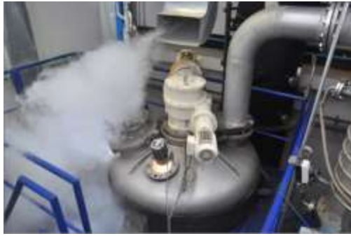
Super-Freeze With Liquid CO2
